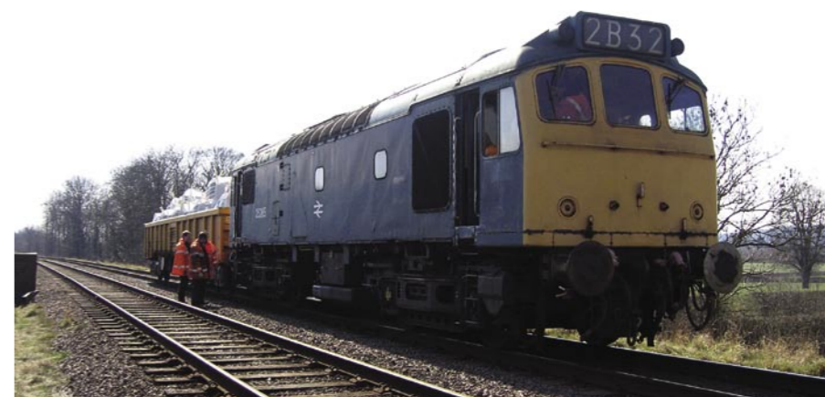
Another GCR test, this time on March 9, 2006. As far as I am aware this was the only time that a Class 25 was used and was due to a fault on 37 255. The wagon concerned is a JNA bogie open box wagon owned by Network Rail. 25 265 is seen coupling up on the slip test section. The Class 25 was not a success, it was not possible to achieve sufficient speed for the higher speed stops due to a field divert problem. In the end we coupled up 37 255 as well and between them they managed the job!
