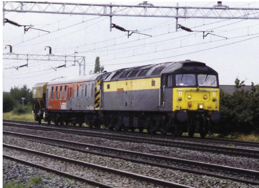
47 976 again, this time entering the test section just north of Crewe. The date is October 5, 1998 and on this occasion we were testing a new disc brake pad material on a single disc per axle CAIB owned PGA aggregate hopper. This was a success and resulted in some new business replacing the competitor's material in a number of single disc per axle applications. Withdrawn in June the following year, Aviemore Castle also ended its days at Wigan CRDC in 2000.
