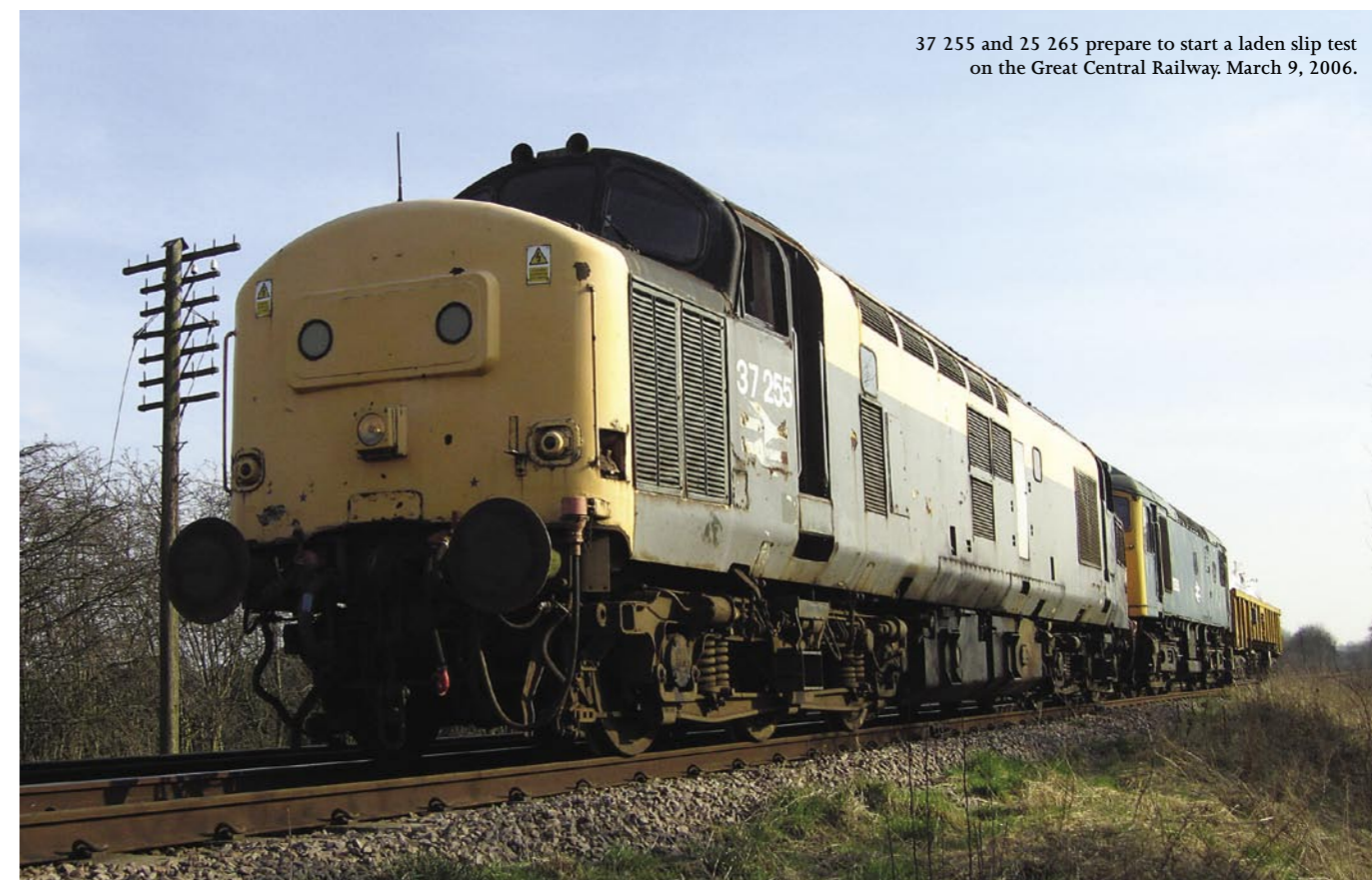
Another GCR test, this time on March 9, 2006. As far as I am aware this was the only time that a Class 25 was used and was due to a fault on 37 255. The wagon concerned is a JNA bogie open box wagon owned by Network Rail. 25 265 is seen coupling up on the slip test section. The Class 25 was not a success, it was not possible to achieve sufficient speed for the higher speed stops due to a field divert problem. In the end we coupled up 37 255 as well and between them they managed the job!
