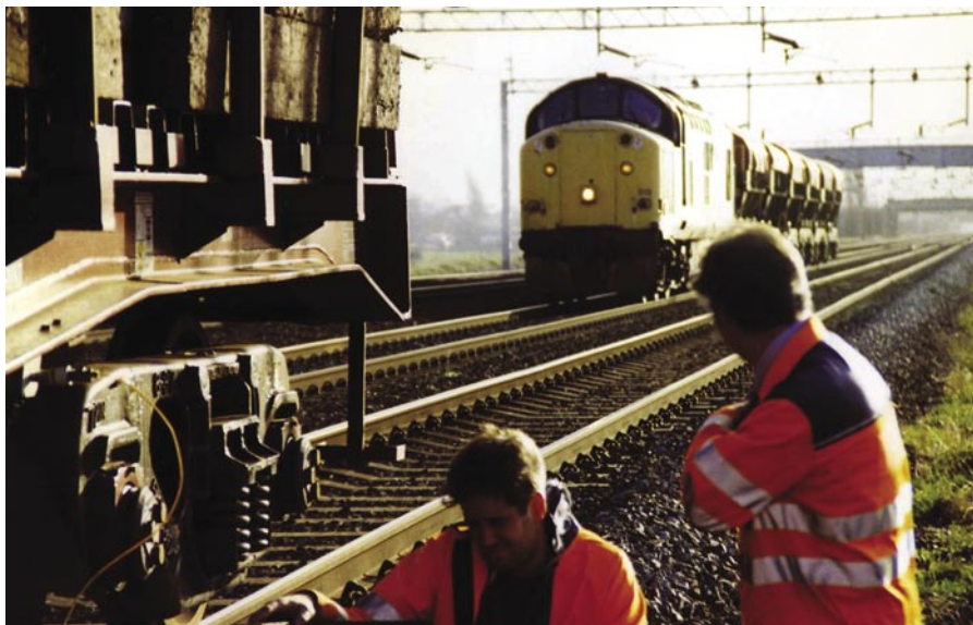
December 10, 1997 near Crewe. This image illustrates the nature of the Crewe/Winsford test location. 37 515 working the Middlewich British Salt to Warrington trip passes Dave Chorley and Chris Wisser who are in the process of carrying out static brake tests on an EWS BAA steel carrier number 900172 that are necessary prior to any slip testing. The presence of running lines alongside the section used for testing made any work other than the actual brake testing itself impossible. In this case the test locomotive was 47 976.
