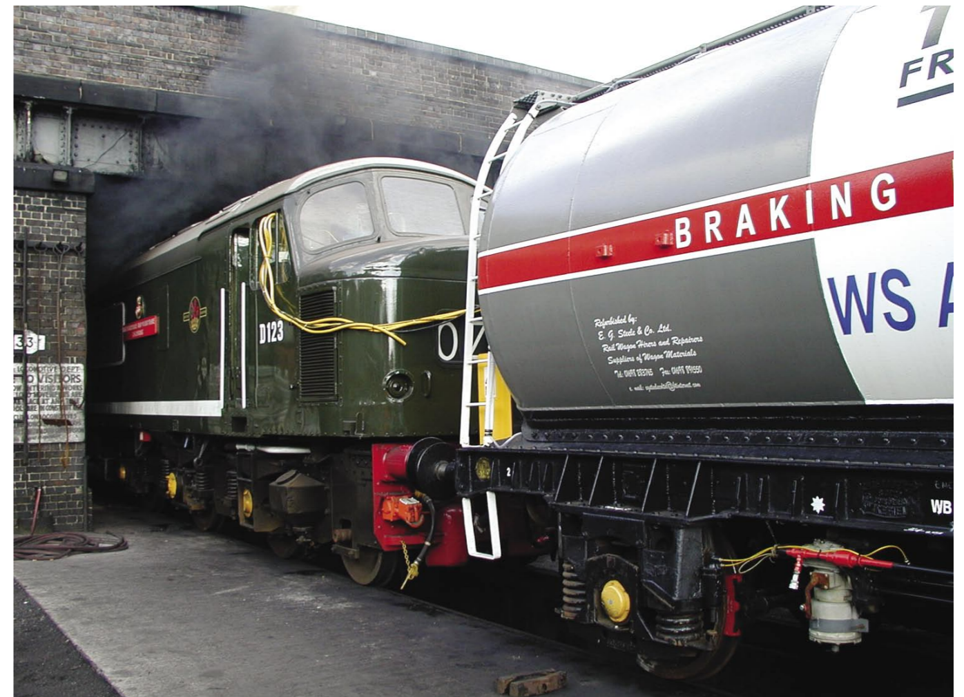
March 13, 2001, preparing for the first slip tests to be conducted on the Great Central Railway. Various cables and pipes associated with the slip coupling operation can be seen running out of the back cab of D123. On this occasion we were testing a cast iron block replacement material and had purchased a redundant two-axle tank wagon from E G Steele to use for a variety of tests.
