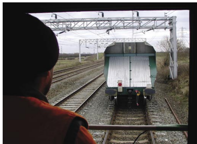
ABOVE LEFT: Crewe/Winsford January 12, 2001 and this is the view from the rear of Test Car 2 and Chris Doleman has just slipped HHA coal hopper 370001. In this case the test train locomotive was 86 632 with 66 602 to pull-back. This was one of the few tests that we failed, the maximum stopping distance recorded being well in excess of target. Eventually, an issue surrounding the lateral movement of the TF25 bogie primary suspension resulting in a reduction in brake block application force was diagnosed and the repeat test following modification was a complete success.
