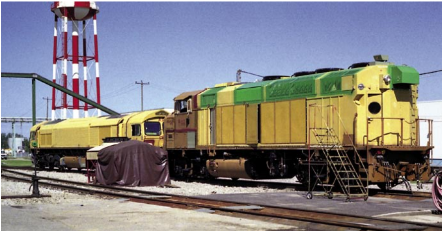
LEFT: In August 1990 Brian went to the EMD works in London Ontario to monitor progress in the construction and testing of the four Class 59/1 locomotives then being built for ARC Southern. In this view 59 102 is seen alongside a diesel electric locomotive being supplied to the Government of Ontario Railroad. Both locos are in shop primer and it clearly shows the difference in loading gauge between Britain and the North American railroads. Delivered to the UK two months later, 59 102 remains in active service with Mendip Rail Ltd operating out of Whately quarry in Somerset.
